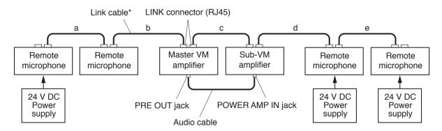
\* TIA/EIA-568A standard Category 5 Shielded Twisted-Pair cable (straight type) Abbreviated to "Cat. 5 STP cable."
