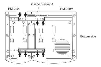
**Note:** If incorrect or loose connection is found between both units, loosen all the bracket fixing screws to disassemble the units and then link them again with the screws.
