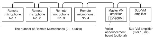
Set the Remote Microphone's Unit number (1-4) using DIP switches No. 1 and No. 2 on the microphone's right side panel. The Unit number may be set regardless of the unit's connection order. (See p. 42 "VM Amplifier's Internal Function Switches.")
