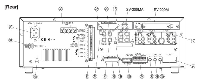
The figure above shows the 230 V AC versions of the VM-2120 and VM-2240. The 120 V AC versions are the same in both appearance and function except the rating indications of the AC inlet (No. 33) and fuse holder (No. 34).
