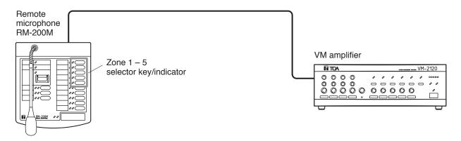
(2) 5 speaker zones with 1 VM amplifier (equipped with the EV-200M Board)
