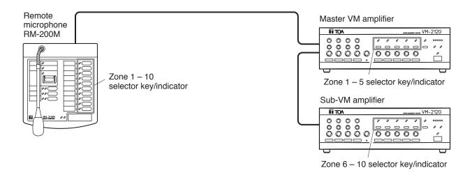
(4) 10 speaker zones with 2 VM amplifiers (equipped with the EV-200M Board)
