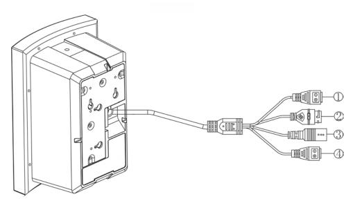
①Amplifier output connector: connector color is black, specification is 3.81-2P, connecting external speaker, when the speaker receives the broadcasting, the same sound can be heard from the speaker. The Rated impedance: $8\Omega$ , the rated output power:30W
