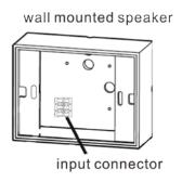
(2) Please refer to the picture to insert the cable into the connector according, and connecting BS -P678IP1 and BS-P678E.
