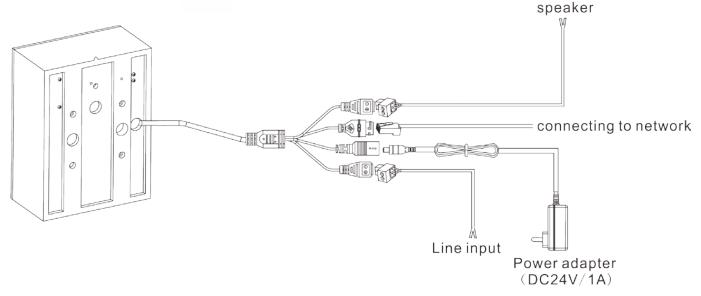
Note: 2P green conntector is for line input, 2P black conntector is for amplifier output.
