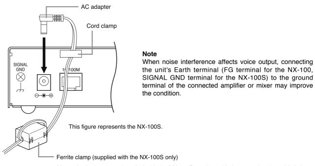
Mount the ferrite clamp (supplied with the NX-100S) on the cable in a way that the cable is looped one turn as illustrated. (This countermeasure is for complying with the CE marking requirements.)
