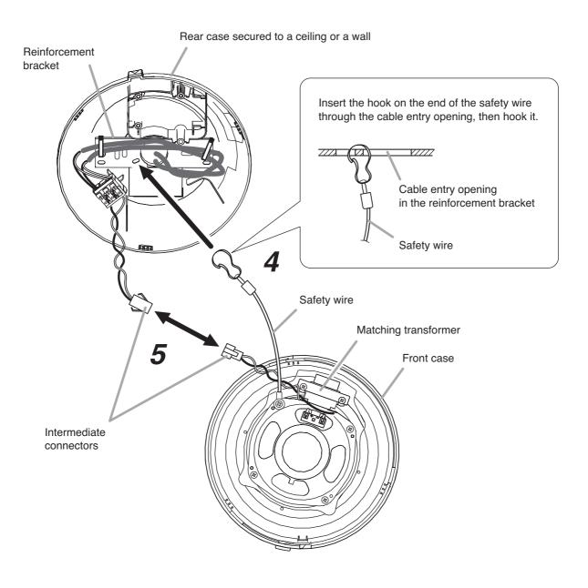
**Step 6.** Secure the front case to the rear case.
