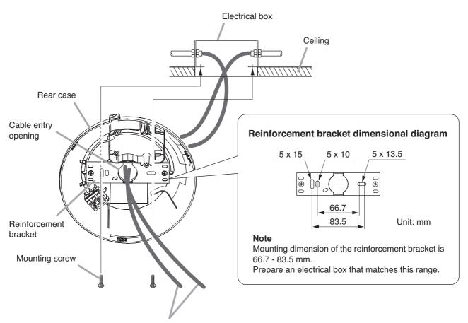
Speaker cables (input line and bridge line)
