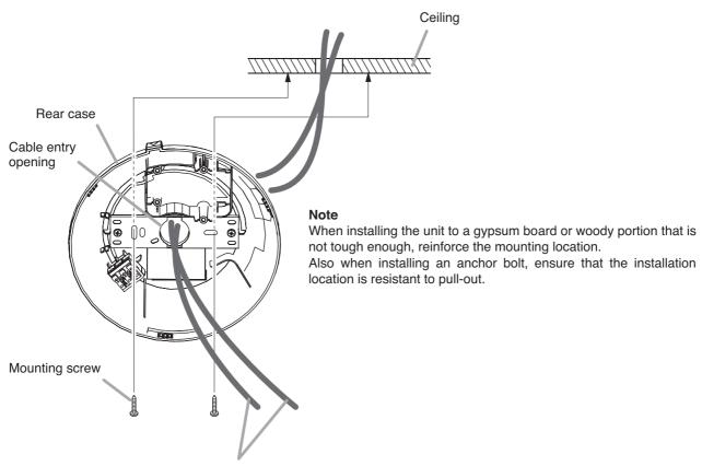
Speaker cables (input line and bridge line)
