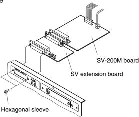
Step 8. Connect the flat cables to the SV extension board.
